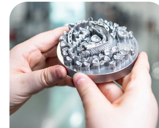
Dental applications, crown and bridges made in CoCr.
