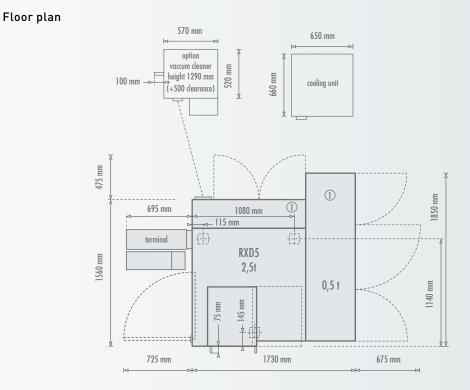
For machine transportation the operator terminal and the electrical cabinet may be taken off.
